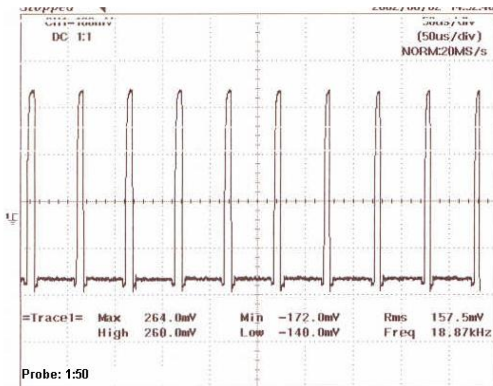
IGBT G, E pole's drive voltage wave ( V_{GE} )
