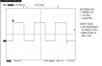
**N.B.** If this signal is absent it may be necessary to replace component Q4 (**fig. 3**).
