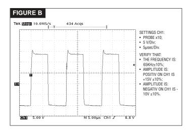
F) Repeat this test on Q5 as well using the differential probe. **N.B.** if the signal is not present, there may be a fault in the IGBT driver circuit (**fig. 4**).
