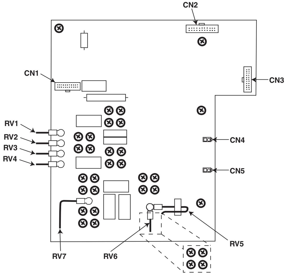
10. Reconnect previously removed leads RV1 thru RV7 to the P.C. board. See Wiring Diagram if necessary.
