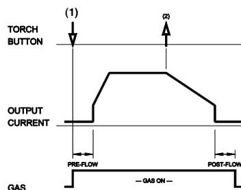
Possible variations of this standard sequence is shown in (2 step diagram 2). It is possible to press and hold the TIG torch trigger a second time during downslope to restart. After the trigger is pressed the output current will increase to the welding current. This operation is shown in (2 step diagram 2).
