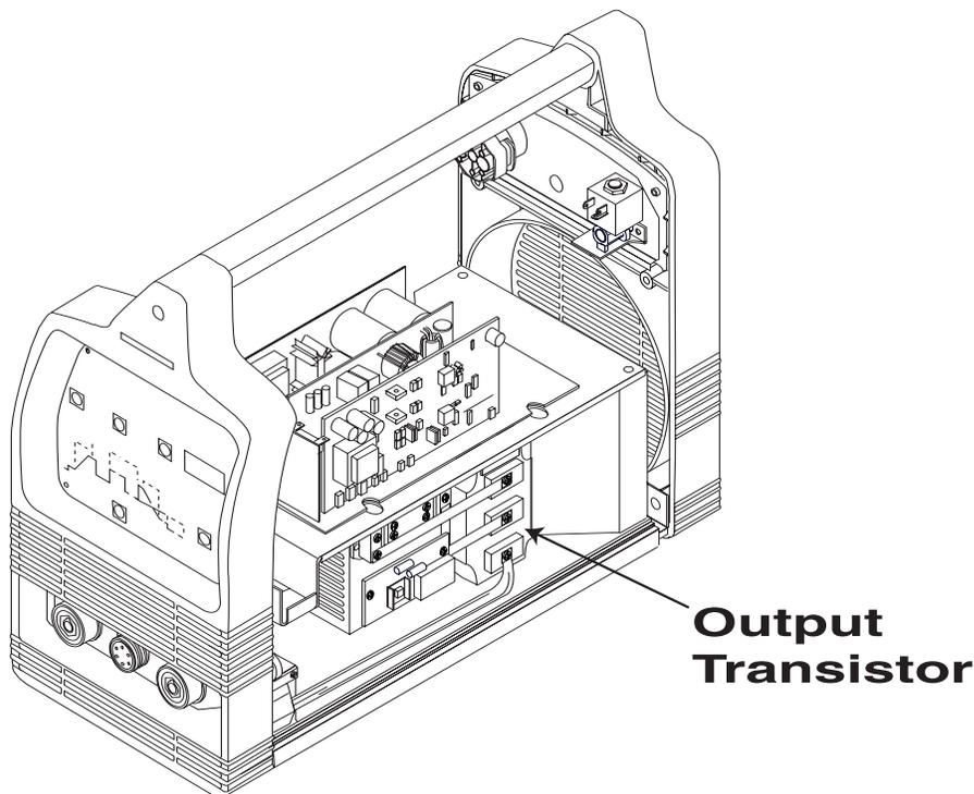
5. Disconnect plug CN1 from the output transistor. **See Figure F.37.**
