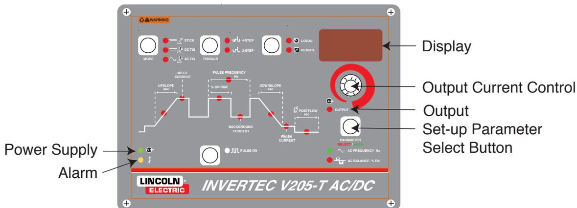
The front panel controls the status of the equipment and shows it to the operator via the LED's and the display. Immediately after switch-on of the equipment, the front panel executes an autotest operation, all LED's will light up and the display shows "200" as a check.
