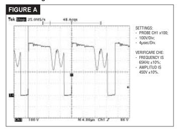
**N.B.** if no signal is present, it may be necessary to replace the integrated circuit U2 (**fig. 3**).
